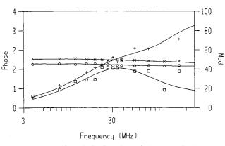
FIGURE 6: Dynamic polarization data of the W15 single mutant with and without fructose-6-P. The upper curves are the data for W15 alone (+, differential phase angle; ×, modulation ratio of perpendicular to parallel polarized component), and the lower curves are the data for W15 in the presence of 30 mM Fru-6-P ( $\square$ , differential phase angle;  $\bigcirc$ , modulation ratio). Solid lines represent fits to the data.
